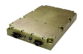
The Apollotek APK8769-HA incorporates a 2.2 to 2.4 GHz or 1.7 to 1.9 GHz Radio Receiver with an integral Bit Synchroniser and is one of the Apollotek range of USB controlled Test Instrumentation products which are designed for Pulse Code Modulation system checkout and evaluation applications.
