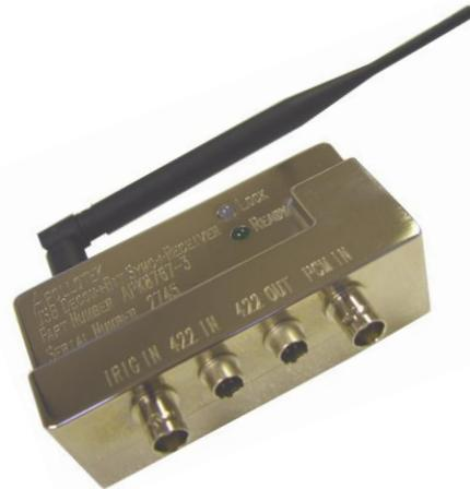
The Apollotek APK8767-3 is a Multi-Function PCM/FM and SOQPSK Telemetry Receiver, Bit Synchroniser and Decommulator. The APK8767-3 is one of a series of Apollotek unique USB products designed for Telemetry, PCM Flight Test Instrumentation system checkout, test and evaluation and Data Link applications. The Unit is packaged into an aerospace grade aluminium housing machined from solid to enable the unit to be used in both ground based and airborne applications.
